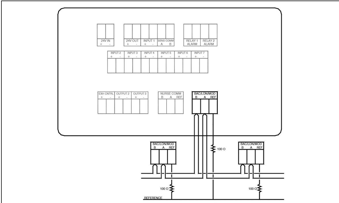
**Figure 33. Optional Modbus and BACnet MS/TP Communications Wiring to Model RPM10/RPM20**
