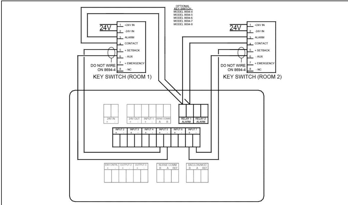
**Figure 29. Optional Key Switch Wiring to Model RPM10/RPM20**
