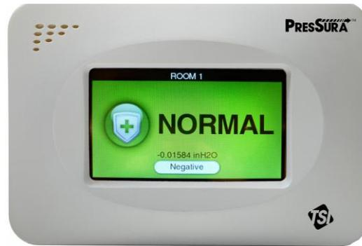
Figure 4. PresSura Room Pressure Monitor
