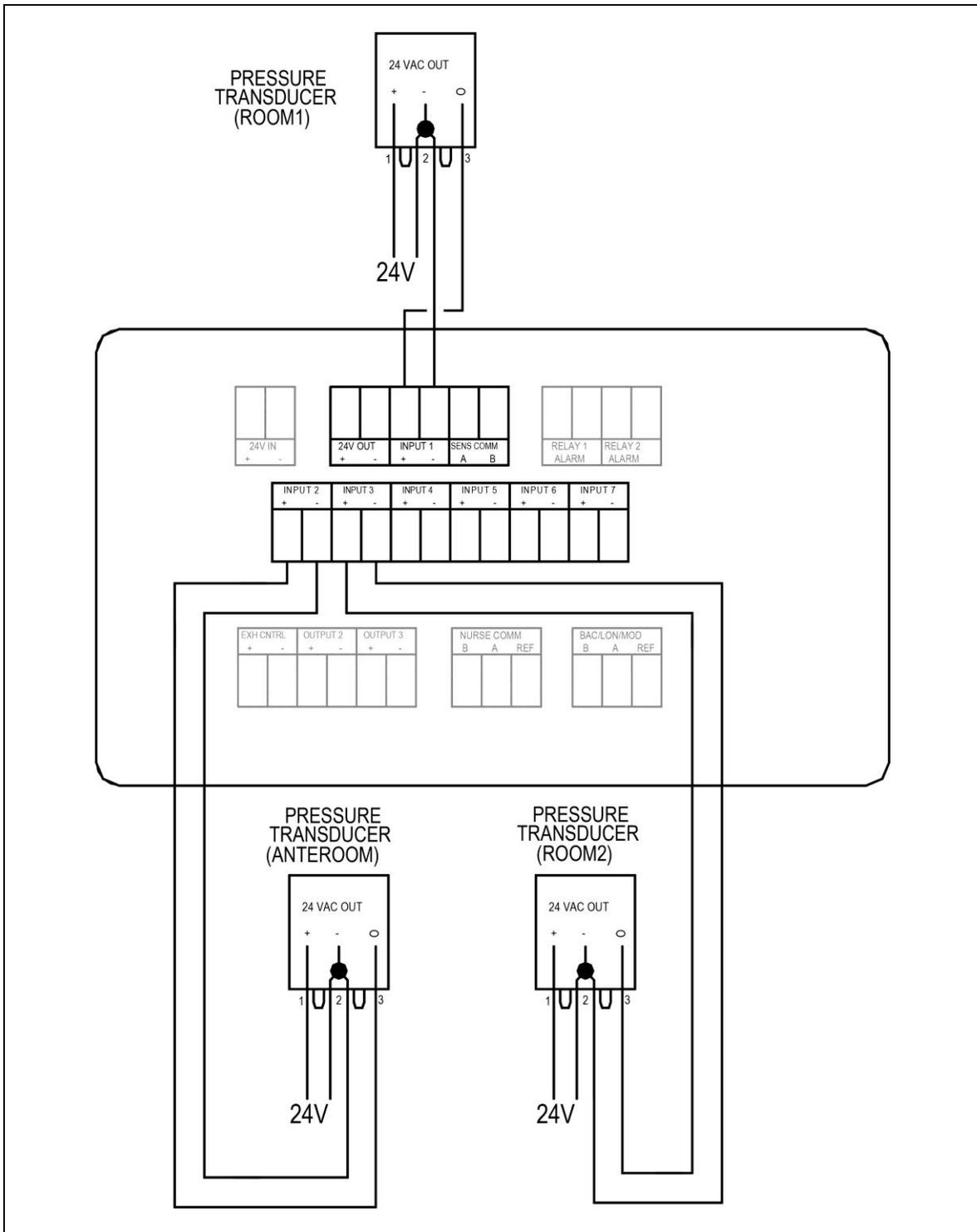
**Figure 20. Pressure Transducer Sensors Wiring to Model RPM10/RPM20**
