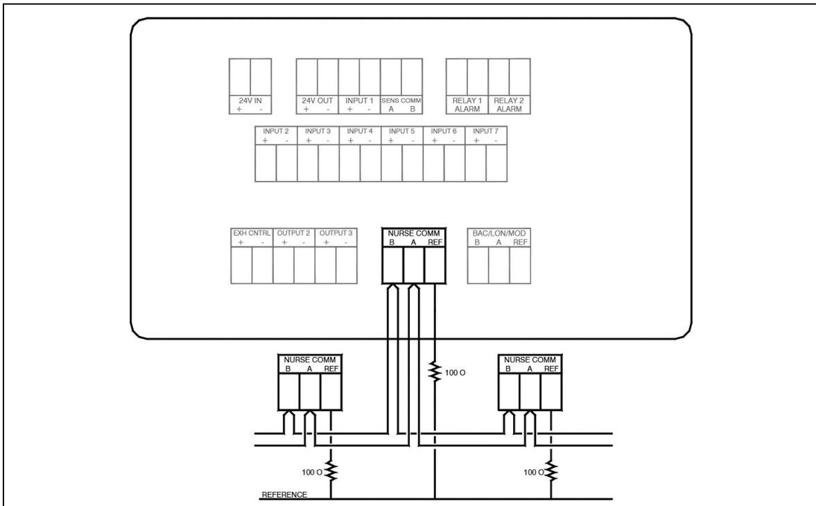
Figure 32. Optional Nurses Station Communications Wiring to Model RPM10/RPM20
