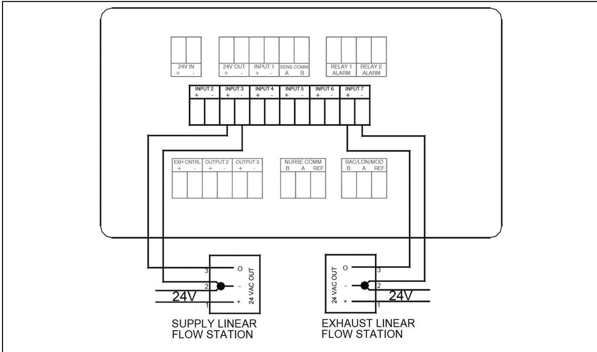
**Figure 23. Optional Supply/Exhaust Linear Flow Station Wiring to Model RPM10/RPM20**
