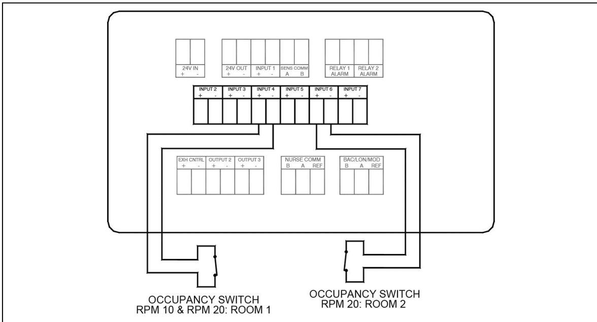
**Figure 27. Optional Occupancy Sensor Wiring to Model RPM10/RPM20**
