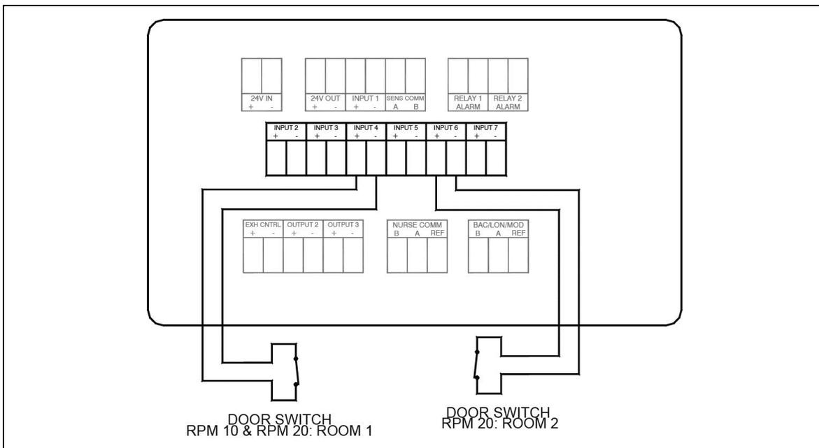
Figure 26. Optional Door Switch Wiring to Model RPM10/RPM20
