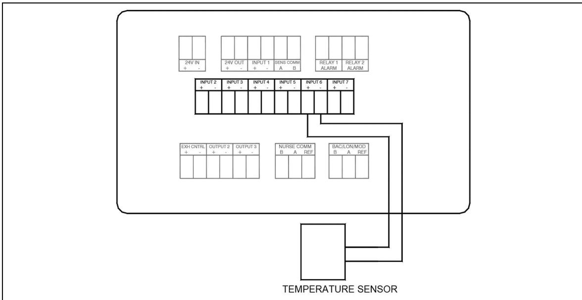
**Figure 28. Optional Temperature Sensor Wiring to Model RPM20**
