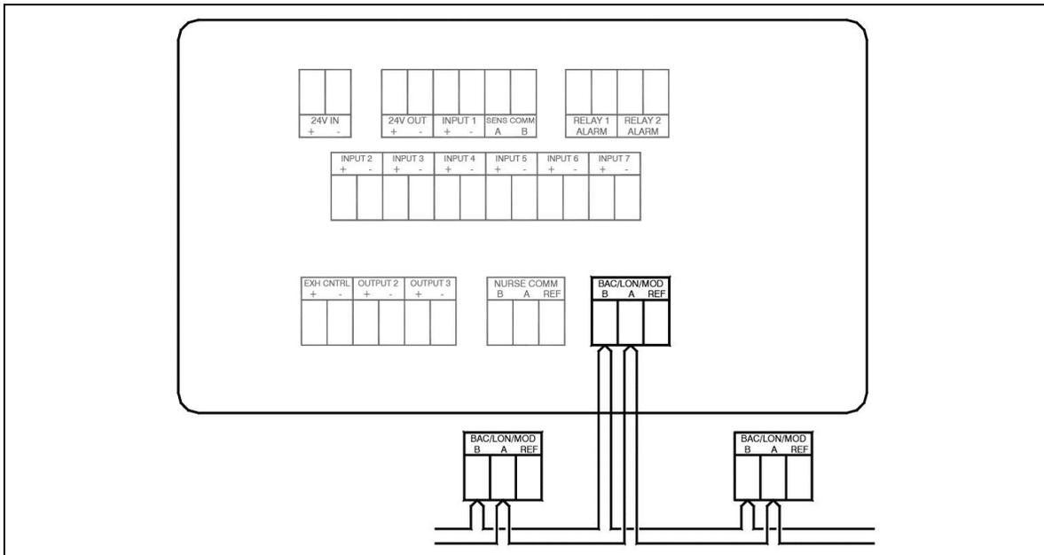
**Figure 34. Optional LONworks Communications Wiring to Model RPM20-LON**
