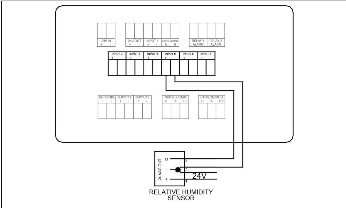
Figure 31. Optional Relative Humidity Sensor Wiring to Model RPM20
