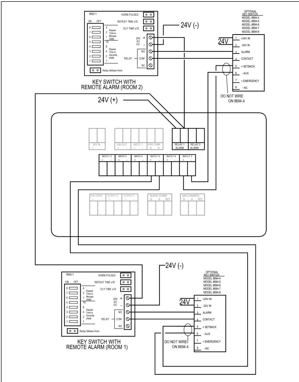
Figure 30. Optional Key Switch with Remote Alarm Wiring to Model RPM10/RPM20
